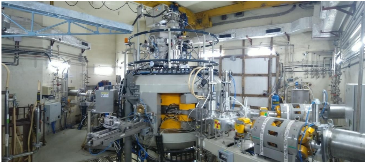
Figure 1: 30 MeV Medical Cyclotron at Chalkgaria campus of VECC Kolkata.
