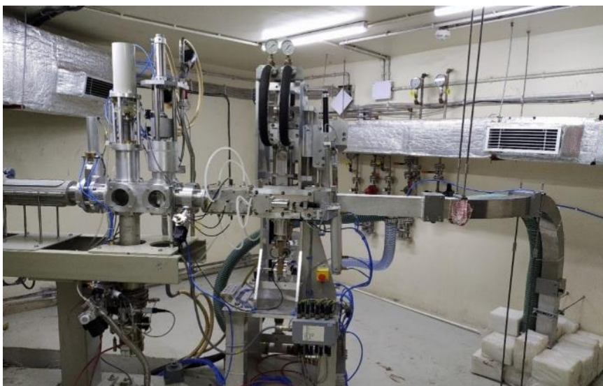
Figure 2: Solid target irradiation system and pneumatic transfer system.
